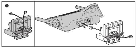
**3** Insert the hooks on the wall mounting adaptor into the holes (**(A)**) and (**(B)**) on the base unit.
